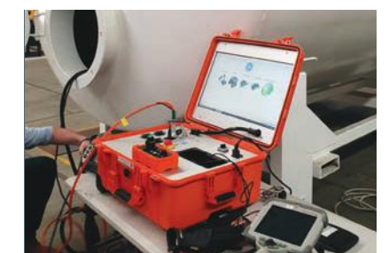
Remote Digital Visual Inspection
